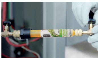
Charge inline with refrigerant
