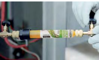
Charge inline with refrigerant
