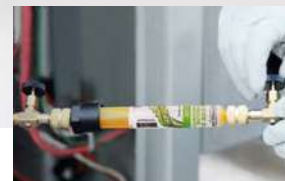
Charge inline with refrigerant
