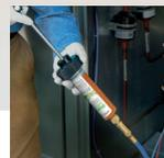
Inject dye with a turn of the handle.
